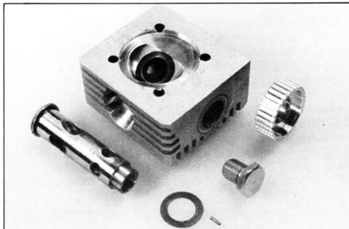
Webra's highly unusual cylinder head and rotary valve assembly. Rotary valve is of chromed brass. Toothed timing wheel is aluminum.
