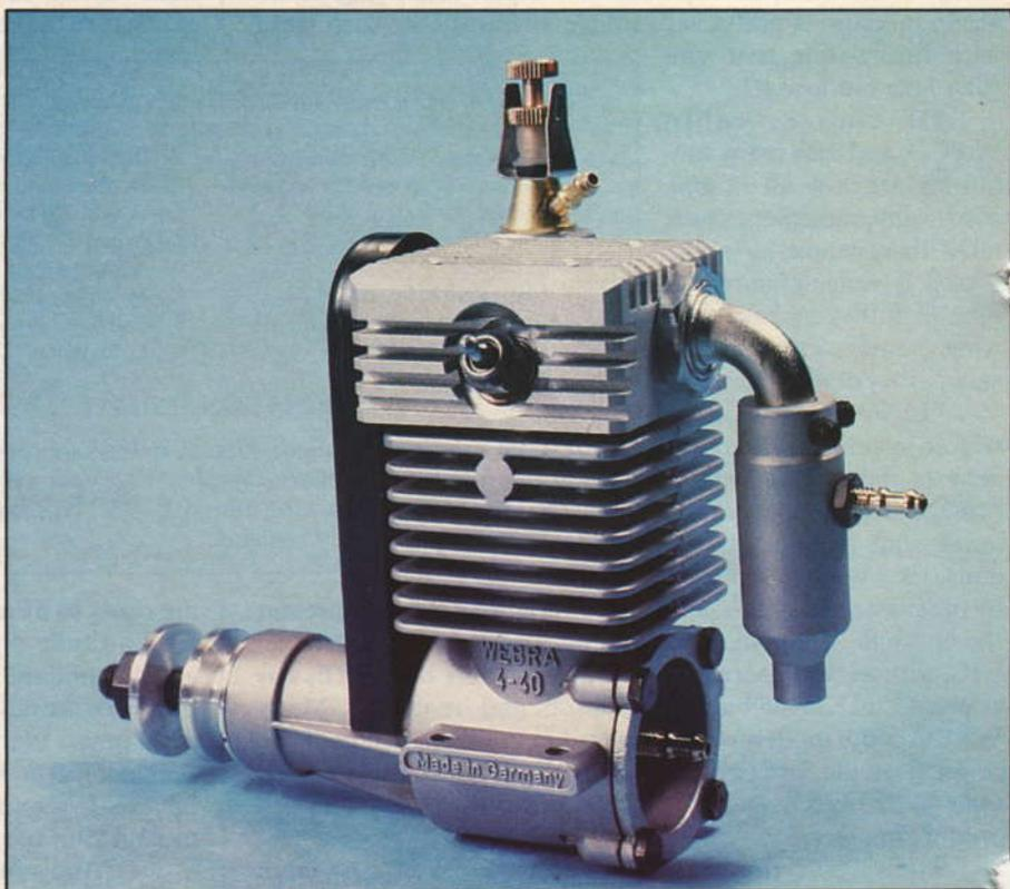
Engine comes complete with muffler, which also provides pressure take-off for fuel tank. Fitting in backplate is crankcase breather.
