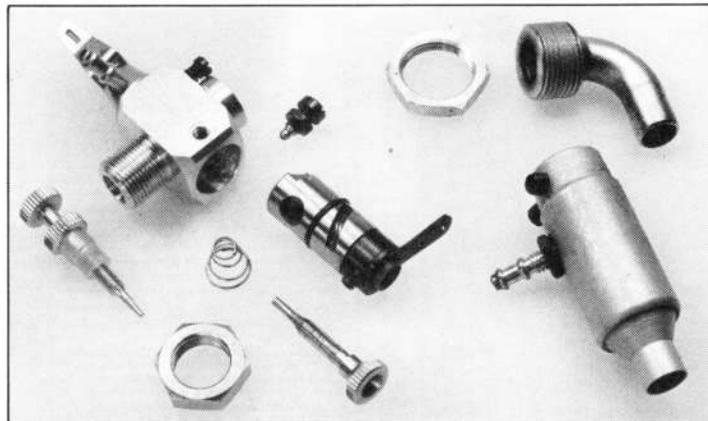
Carburetor parts, left, showing two needles and O-ringed throttle barrel. Exhaust elbow and muffler assembly on right.
