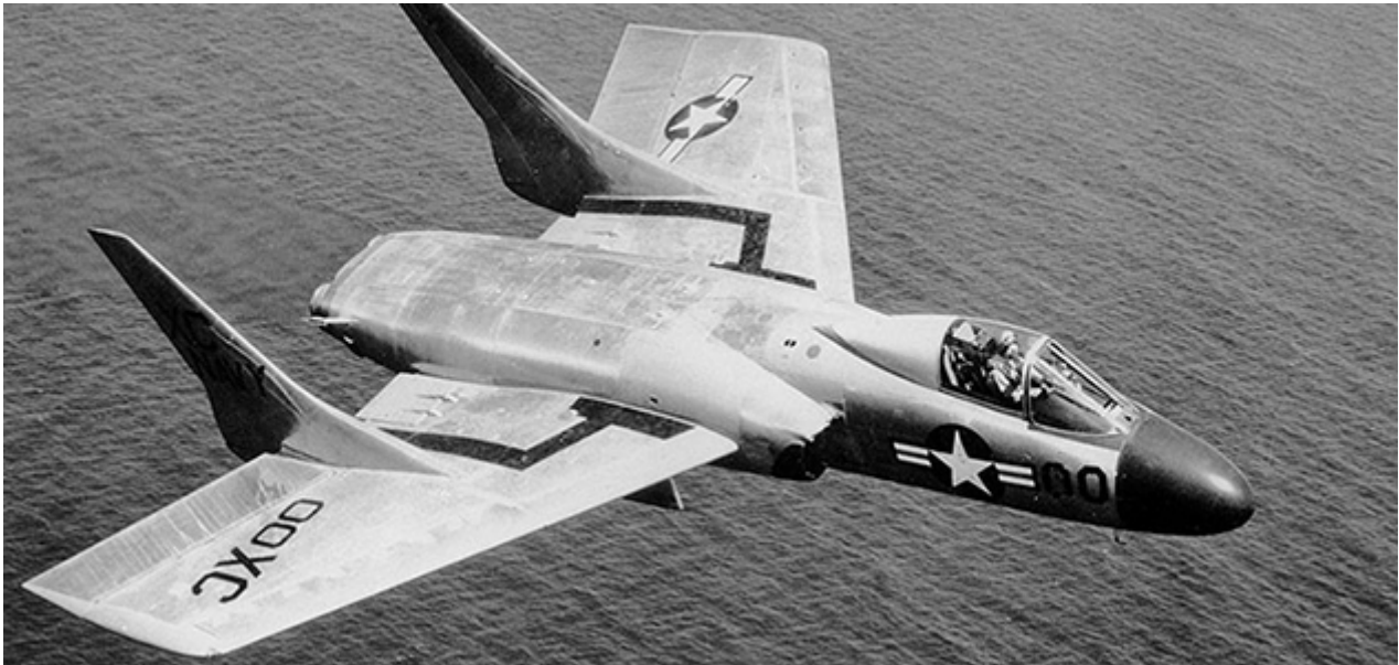
The “Gutless Cutless” earned its nickname primarily from its underpowered engines. A Vought F7U-3 in May 1953.
