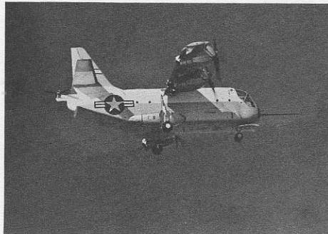
again tilted 10 degrees, the XC-142A rolled to taxi speed—without using brakes—within 1000 feet.
